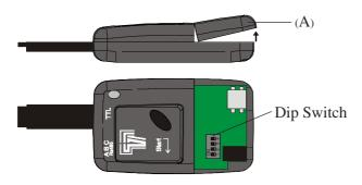
Raise the cover (A). It will be easy to identify the dip switches.
