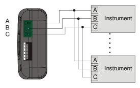
power supply (the instrument must be powered) RS 485 connectionCollegamento interfaccia RS 485
