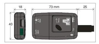
TTL Connector: JST S 5B-PH-KL - 2 mm
